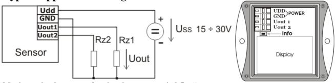
Maximum load current of each voltage output is 0.5 mA
